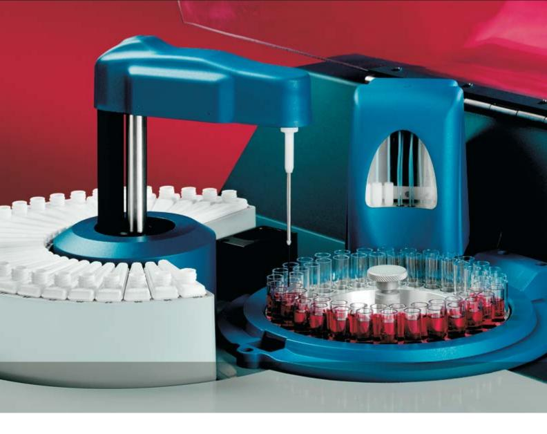
**Tests**: All the analyses regarding a spectrophotometric determination can be automatized.
